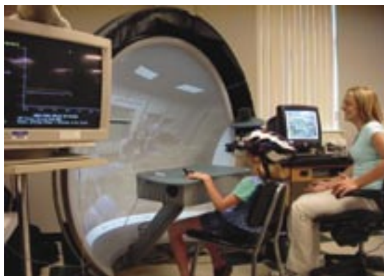
FIGURE 4. Virtual Classroom displayed on an Elumens VisionStation® with eye and head tracking
